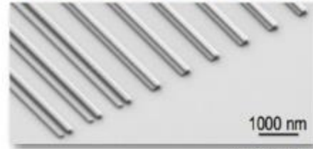
SEM image of two layer lithography with negative resist (HSQ)
